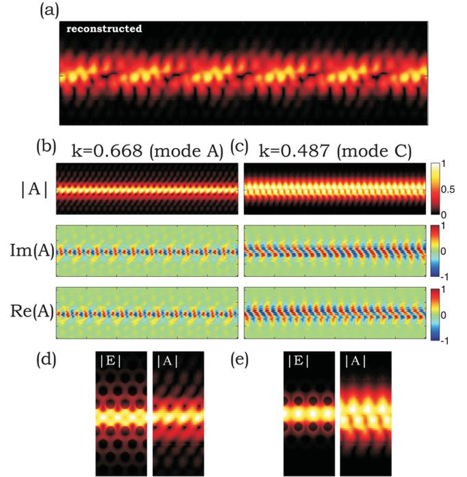
FIG. 3. (Color online) (a) Reconstructed amplitude for Fig. 2(a) using Bloch modes  $m=4$  and  $m=5$  only. (b and c) Amplitude, imaginary part, and real part for both Bloch modes. (d and e) Comparison between calculated  $\langle |E| \rangle$  (left) and reconstructed  $|A|$  (right).
