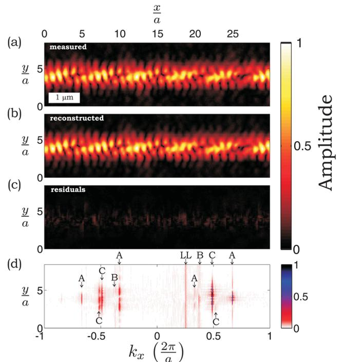
FIG. 2. (Color online) (a) Measured amplitude for a photonic-crystal waveguide at  $931.6 \pm 0.1$  nm. (b) Fitted amplitude using seven reconstructed Bloch modes over 30 unit cells. (c) Residual amplitude. (d) Amplitude coefficients of the spatial Fourier transforms of the measured near-field pattern. Labels correspond to those in Fig. 1(b).
