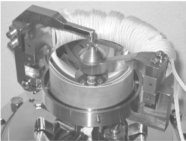
FIG. 3. The SNOM with spherical mirror. Behind the mirror is the semicircular coil core made of pure iron. On the right hand side, the magnetic field is piped under the sample, on the left side over the sample.
